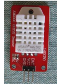
DHT22 Pinout Pin 1: VCC (3V to 5.5V) Pin 2: Data Pin 3: Not Connected Pin 4: Ground
